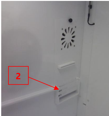
Figure 92: Water Tank fill port
