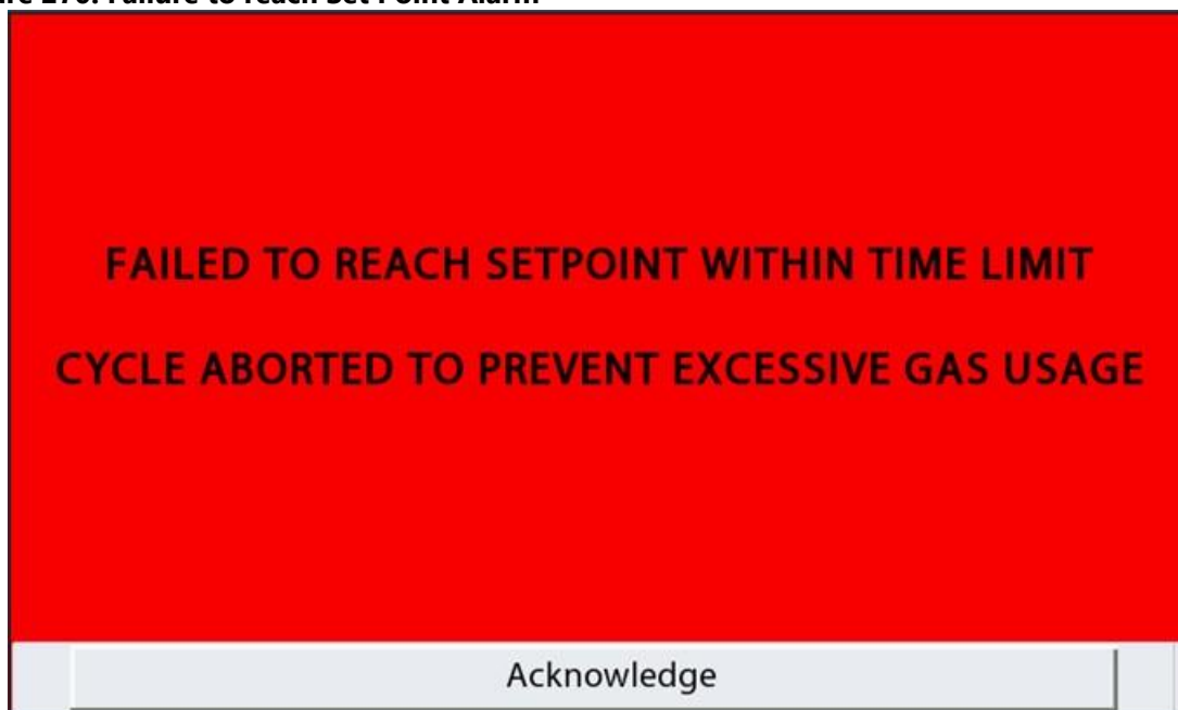
Figure 270: Failure to reach Set Point Alarm
